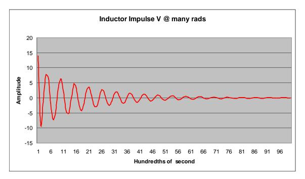
To repeat, note that if the factor on  $s^1$  is 0 (means R = 0) then the circuit oscillates at  $\omega = \sqrt{29}$ . Whereas when  $R \neq 0$  the frequency is lower (in this case 2) - and that will be true with all oscillating circuits. When R = 0 the circuit will theoretically oscillate
