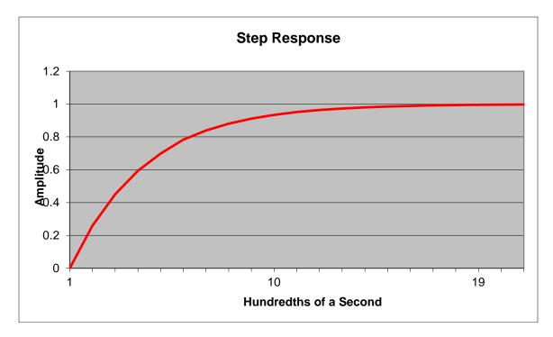
It is interesting to note the relationship between the impulse and unit step response, both mathematically and graphically. But the real significance is that the impulse response uncovers the transient time response of the circuit, and the step response is the circuit response to a DC driver (or, importantly, the DC component of a driver, such as  $f(t) = \sin(\omega t) + cnst$ ).
