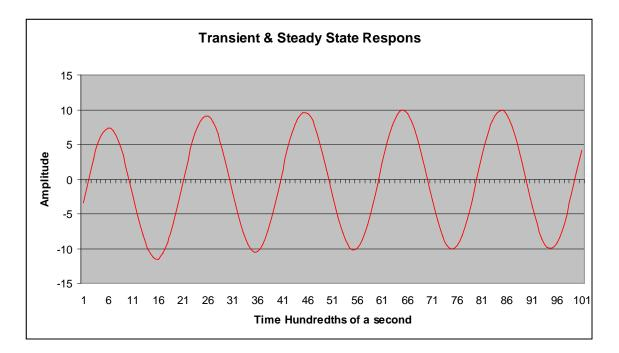
In the above graph the amplitude of the transient portion has been distorted purposefully to better identify its contribution to the output. It should be clear that by the end of the second cycle it has fully disappeared.
