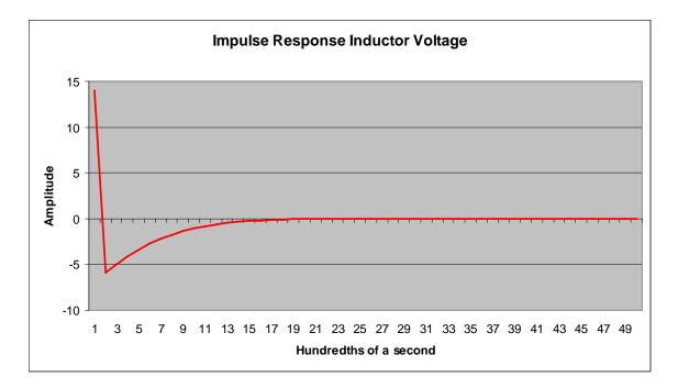
The above figure fairly well captures the effect that  $\delta(t)$  has on the impulse response. To amplify the effect of  $e^{\frac{-Rt}{2L}}$ ,  $\omega_d$  is arbitrarily increased below; simply to illustrate how the exponential decay dominates the impulse response.
